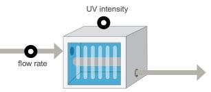
With the UV Intensity Setpoint approach, UVT monitoring is not required on the influent to the UV reactor. However, it is critical to consider the likely water quality of the influent in terms of UVT when selecting the appropriate reactor. An MBR-treated blackwater may have a UVT in the 60-75% range; if a reactor was validated only down to a UVT of 80%, the system will fail to meet the UV intensity setpoint and thus the reactor would not be an appropriate choice.
